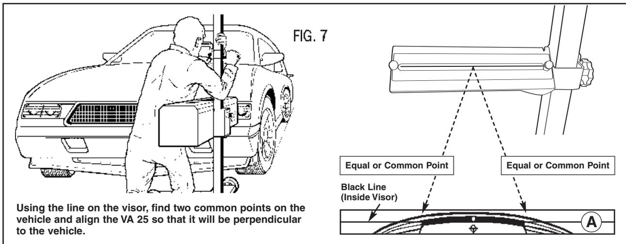
Using the line on the visor, find two common points on the vehicle and align the VA 25 so that it will be perpendicular to the vehicle.
